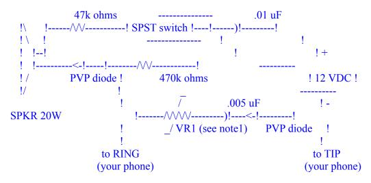
note1 - VR1 is a three position variable resistor, enabling settings equivalent to 100k ohms, 210k ohms, and 320k ohms (all 110k apart).
